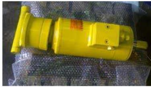
HM9 SWIVEL BOOM LIFT CYLINDERS
