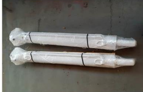
SHORTWALL DA RAM CYLINDERS
