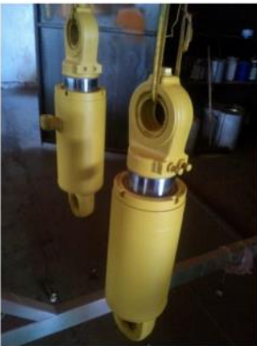
CAT 740B SUSPENSION CYLINDERS
