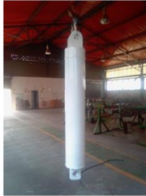
SHORTWALL GATE RAM CYLINDERS
